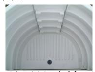
Place drain cap in bottom of well. Connect drain cap to 4" standard pipe then connect pipe to drainage tile system. Then attach the pipe to the wall with metal strapping.
