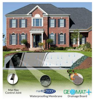
3-Way Foundation Protection: Control. Impermeability. Drainage.
